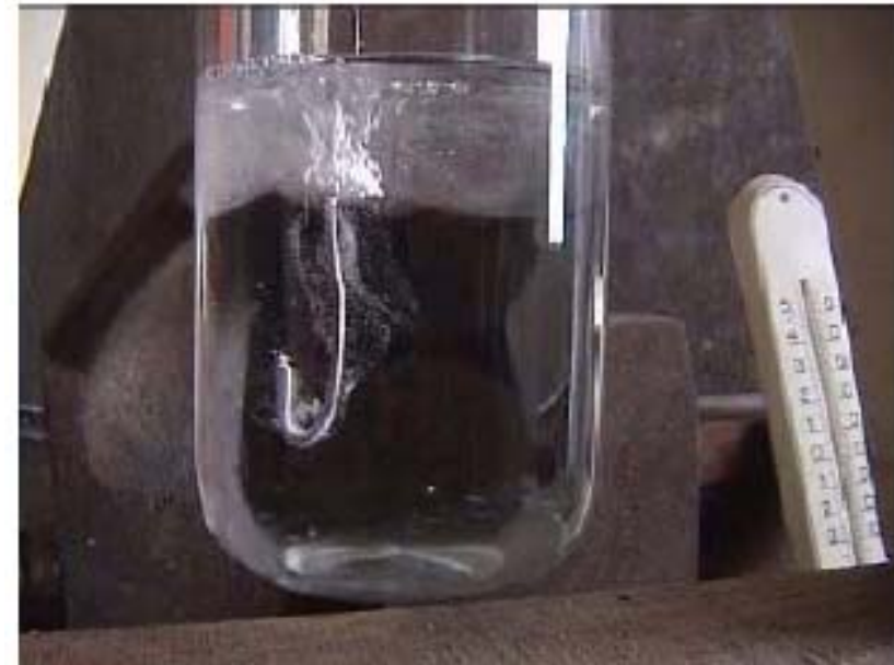
Kinetic experiment of sodium in alkaline solution
